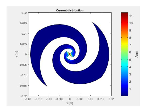
The patch also shows the current distribution of the classic  $\lambda$  / 2 open-open resistor. The two ends of the patch represent an open circuit since the current is at a minimum.
