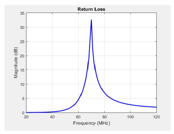
Return loss plots also give the operating bandwidth of the antenna. Antenna bandwidth is the frequency band over which the magnitude of return loss is greater than 10 dB. Use the returnLoss function to calculate the return loss of any antenna in the Antenna Toolbox library.
