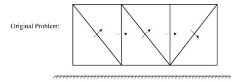
You formulate the problem by considering real and image basis functions. You can show the same problem using image theory or method of images. The interaction matrix is calculated using the interaction between real and image basis functions.
