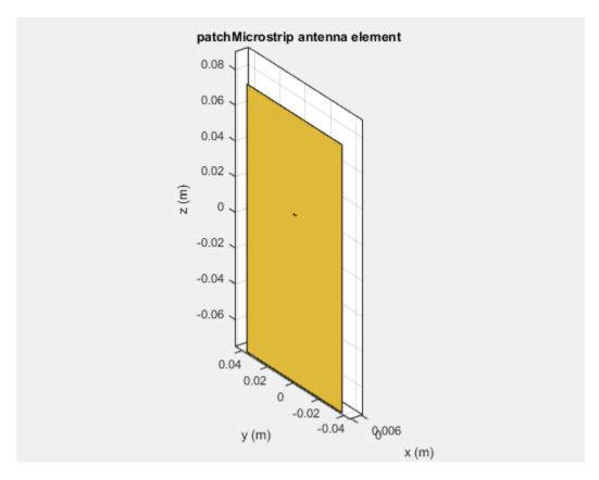
The patch lies behind the ground plane and is not visible. To make the patch visible (in front of the ground plane), rotate the antenna about the negative y-axis.
