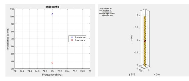
In above example, the dipole is meshed at 75 MHz automatically before calculating the impedance at that value. Use the mesh command to view the meshed dipole. The number of triangles is 44.
